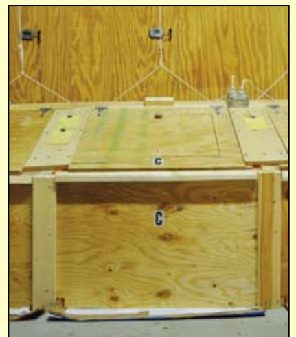
Unit C with the window cover in place. On cool nights the cover fills the window as shown; on days that are not warm enough to remove the cover entirely, it may be slightly offset to provide some ventilation. The electrical outlet on the right of unit C controls the heater panels for units C and D.
